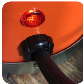
"Power on" indicator light
